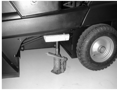
Intake point for the jack (rear wheels)
