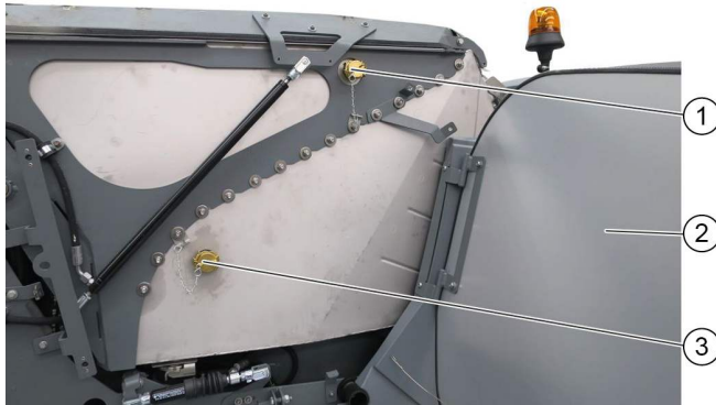
Filling the fresh water tank in a water circulation system
