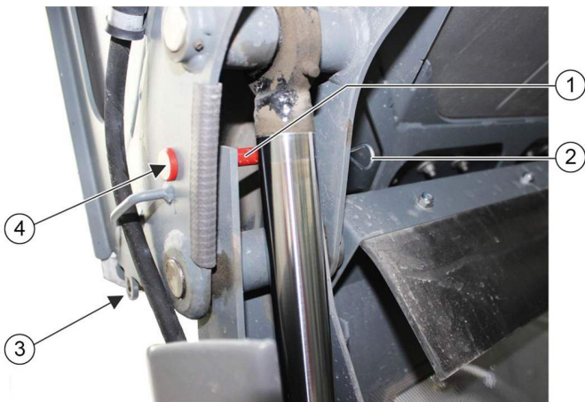
Securing the raised waste container
