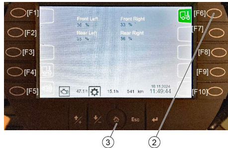
Fig. 73: Activating the loading mode
