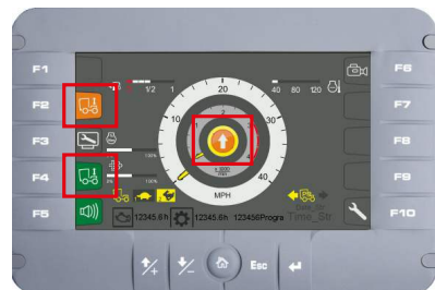
Fig. 84: Terrain mode active when sweeper is in transport mode
