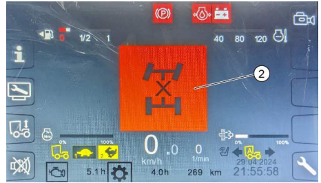
Fig. 80: Differential lock symbol in the multi-function display
