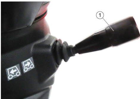
Fig. 67: Travel direction selector switch
