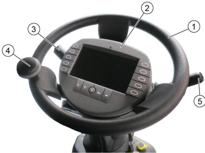
Fig. 29: Steering wheel console with multi-function display
