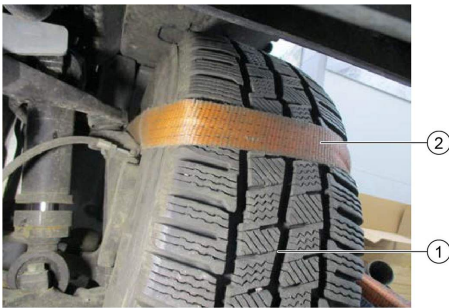
Fig. 98: Lashing strap on front wheel
