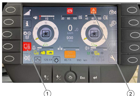
Fig. 77: Fault detection in the event of a fault in the suspension system
