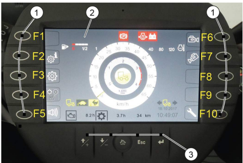
Fig. 34: Buttons on the multifunction display
