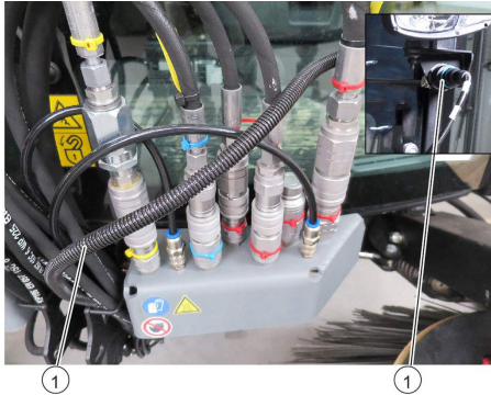
Fig. 14: Front electrical connections for front attachment
