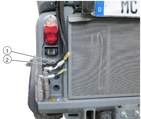
Fig. 15: Rear electrical connections for rear attachment
