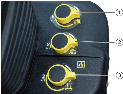
Fig. 61: Dosing knobs for spraying
