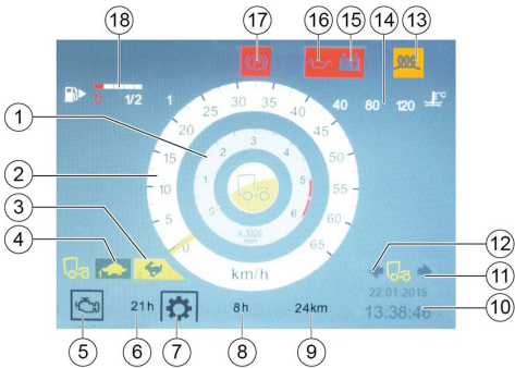
Fig. 36: Multifunction display: Displays in start/transport mode
