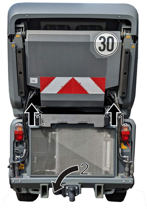
Fig. 123: Removing the radiator protective grille
