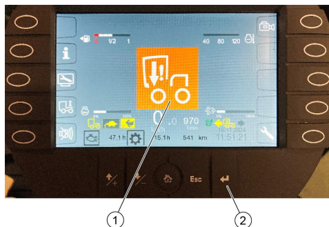
Fig. 74: Warning symbol in the center of the multifunction display
