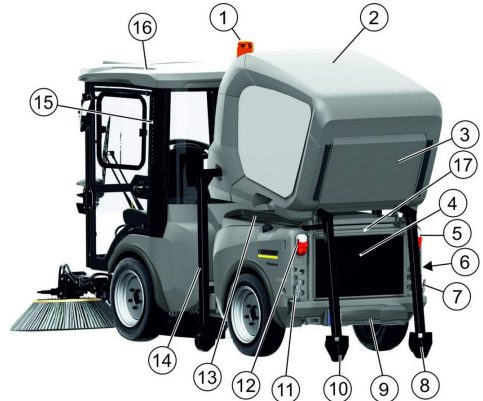
Fig. 7: View with waste container on supports
