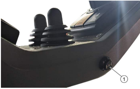
Fig. 79: Differential lock button
