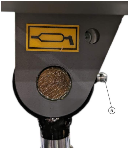
Fig. 106: Mounting frame hydraulic cylinder lubrication point
