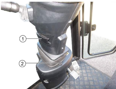
Fig. 66: Steering wheel adjustment on the steering column
