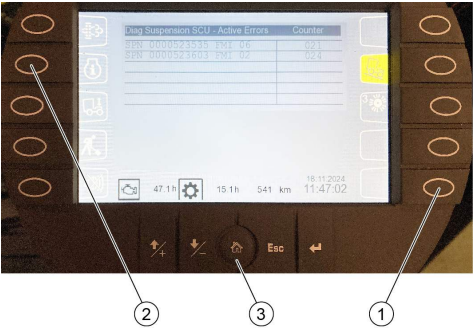
Fig. 78: Suspension system fault codes
