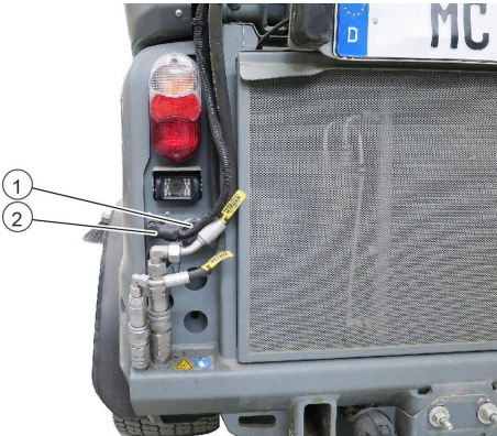
Fig. 56: Rear electrical connections for rear attachment
