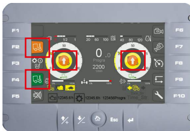
Fig. 83: Terrain mode active when sweeper is in working mode
