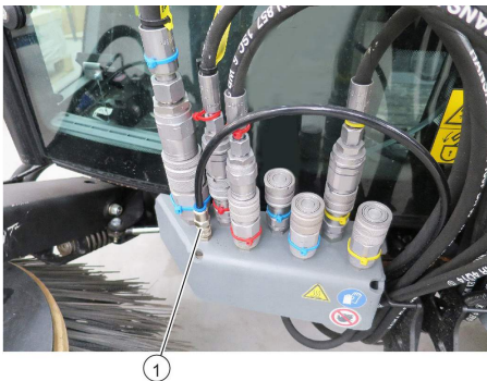
Fig. 16: Front right spray water connections
